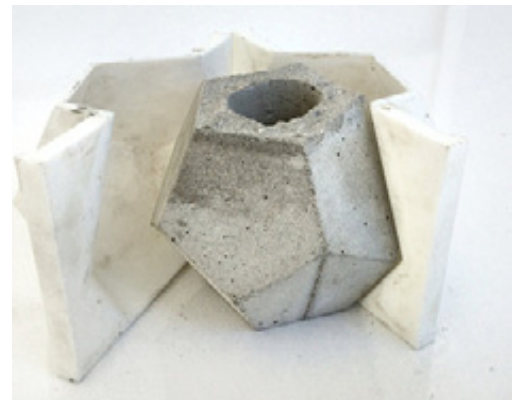
(Fig. 12) 3d printed plastic mold to create concrete form. A similar system would be used for the information artefact
